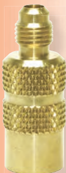
92863 R410A Mini-Split Adaptor 5/16" [1/2"-20] Female w/ Depressor x 1/4" Male w/ valve core
