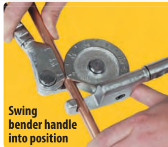
Bend tubing to desired angle
